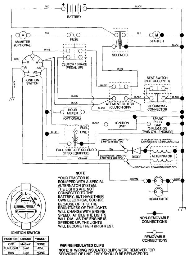
SERVICING OF UNIT, THEY SHOULD BE REPLACED TO PROPERLY SECURE YOUR WIRING.
